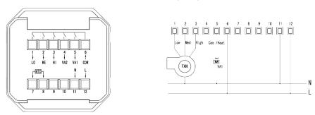
LCF Touch Standard –wiring diagram for 4-pipe fan coil
