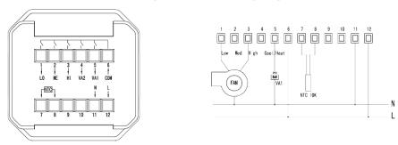
LCF Touch Standard – Manual mode wiring diagram for 2-pipe fan coil
